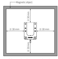
• Install the switch to the position where the center of the switch and the target be exactly horizontal and vertical.
